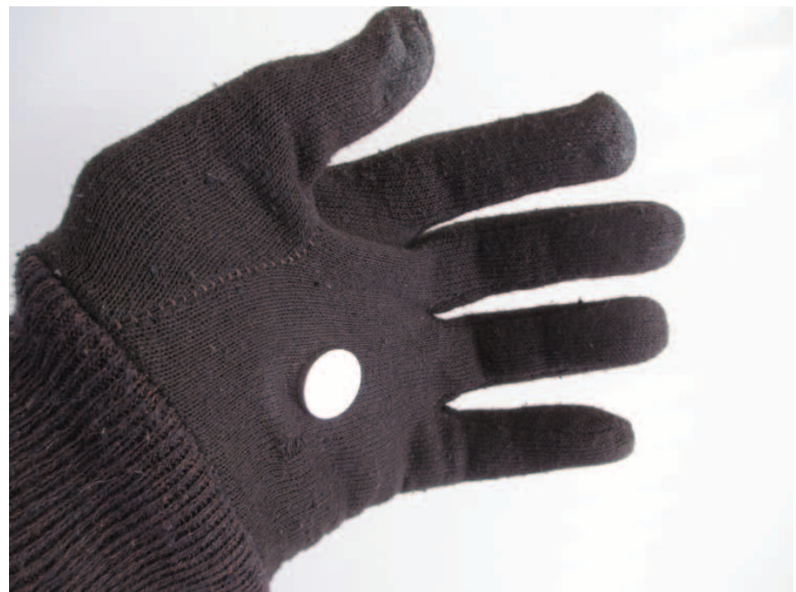
Fig. 3. A sound glove with neodymium magnet attached. (© Jess Rowland)
