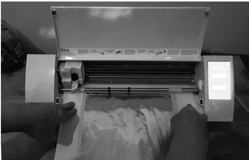
Figure 9.2 Feeding a foil sheet with adhesive backing, placed on a white cutter mat, into the craft cutter.
